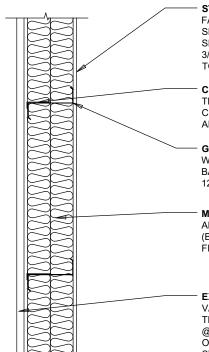
STEEL LINER: PANELS FABRICATED FROM MINIMUM 24 Gauge (0.61mm) THICK SHEET, FASTENED TO GIRTS BY 1" (25mm) LONG (USE 1 1/2" (38mm) LONG @ CLOSURE LOCATIONS) SELF DRILL TEK SCREWS SPACED MAXIMUM 12" (305mm) ON CENTER. SIDE LAP JOINTS SEALED WITH 1/8" x 1/2" (3 x 13mm) FIELD APPLIED TAPE SEALER AND SECURED WITH 3/4" (19mm) LONG STITCH SCREWS 12" (305mm) ON CENTER. ENDS AND SPLICES TO BE SEALED WITH 1/8" x 1/2" (3X13mm) FIELD APPLIED TAPE SEALER TO FORM AIR BARRIER.
