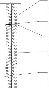
STEEL LINER: PANELS FABRICATED FROM MINIMUM 24 Gauge (0.61mm) THICK SHEET, FASTENED TO GIRTS BY 1" (25mm) LONG (USE 1 1/2" (38mm) LONG @ CLOSURE LOCATIONS) SELF DRILL TEK SCREWS SPACED MAXIMUM 12" (305mm) ON CENTER. SIDE LAP JOINTS SEALED WITH 1/8" x 1/2" (3 x 13mm) FIELD APPLIED TAPE SEALER AND SECURED WITH 3/4" (19mm) LONG STITCH SCREWS 12" (305mm) ON CENTER. ENDS AND SPLICES TO BE SEALED WITH 1/8" x 1/2" (3X13mm) FIELD APPLIED TAPE SEALER TO FORM AIR BARRIER.
